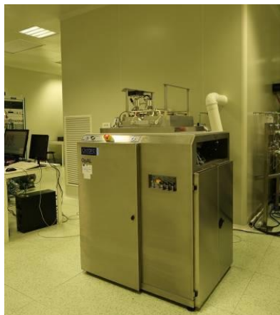
Fig. 4 A picture taken from the clean room of the CENASIC experimental infrastructure (the new centre within IMT), showing an equipment for Atomic Layer Deposition (ALD)
