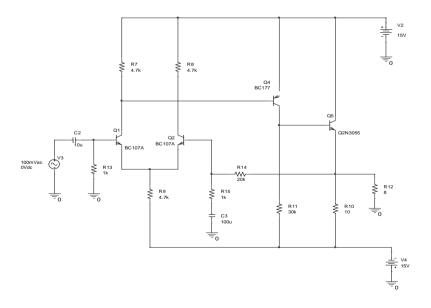
the approximate transfer function that describes the essential behavior. For the integrated audio amplifier below, the system finds the transfer function too "noisy", and proposes to "clean" it, by insertion of RC series group in parallel to  $R_{14}$ ; further it verifies whether the capacitance can be integrated.
